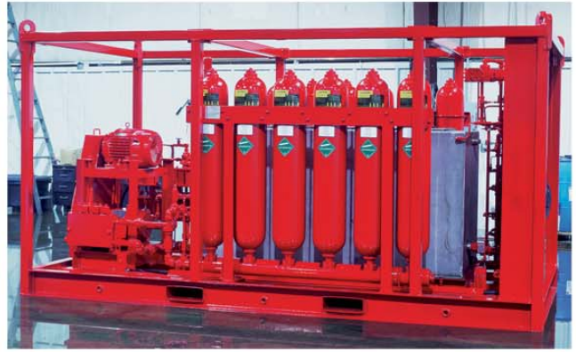
Here, a Plunger Pump is packaged in a 10,000 psi (690 bar) blowout preventer control skid for offshore application.
